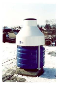
The MRW500 is a rain gauge with weighing principle of measuring precipitation, with a catching area of 500 cm² and a resolution of 0.1 mm of precipitation. It is designed for measuring liquid and solid precipitation. The basic element for measuring is a strain gauge connected to the control electronics, which continuously evaluate the measurements and control other parts of the rain gauge.
