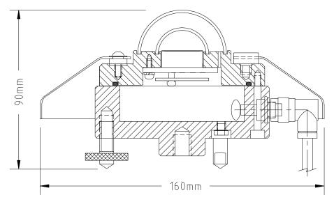
Carbon nanotube (CNT) blackened sensor surface has flat spectral response and excellent stability.
